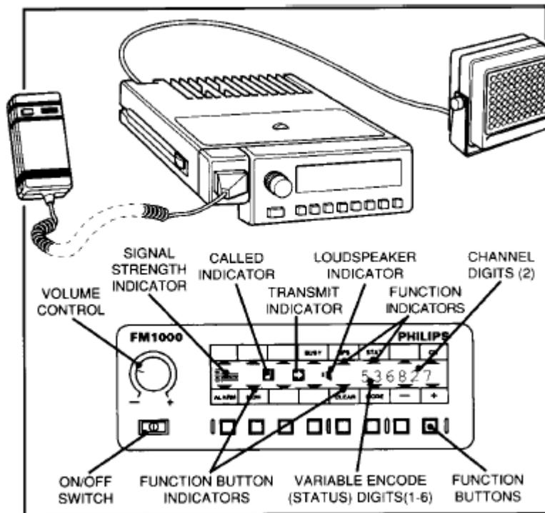
**Fig 70:** THE PHILIPS FM1100 MRT BASE SET RADIO (Carry frame not shown)
